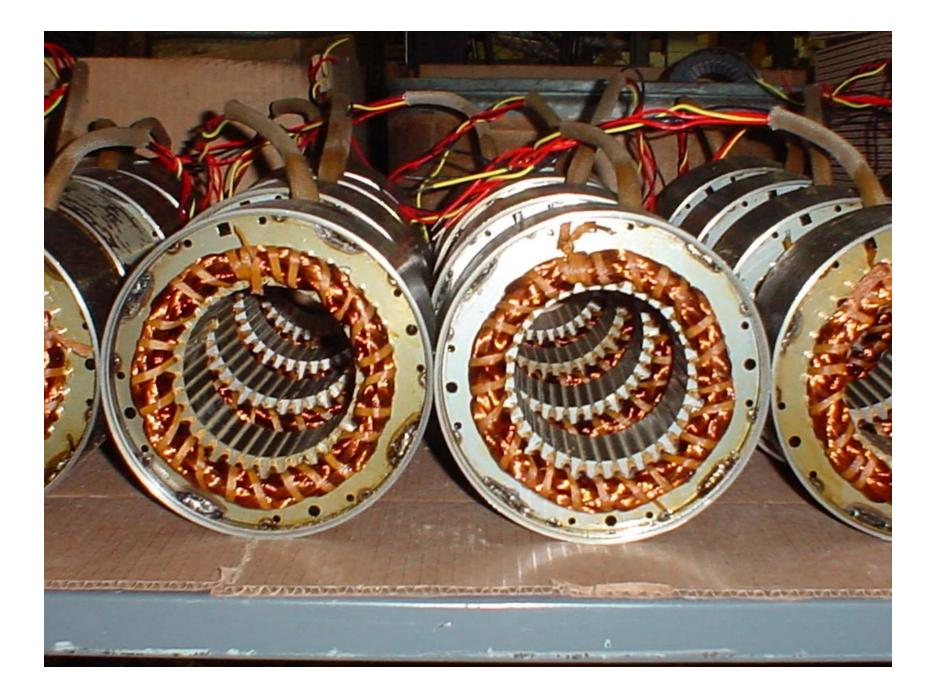
All laminations are stacked utilizing designed stacking tools and fixtures.
