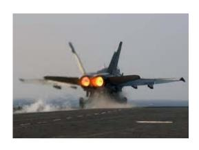
An afterburner is an additional component added to jet engines, primarily those on military supersonic aircraft. Its purpose is to provide a temporary increase in thrust, both for supersonic flight and for takeoff. On military aircraft this extra thrust is useful for combat situations.
