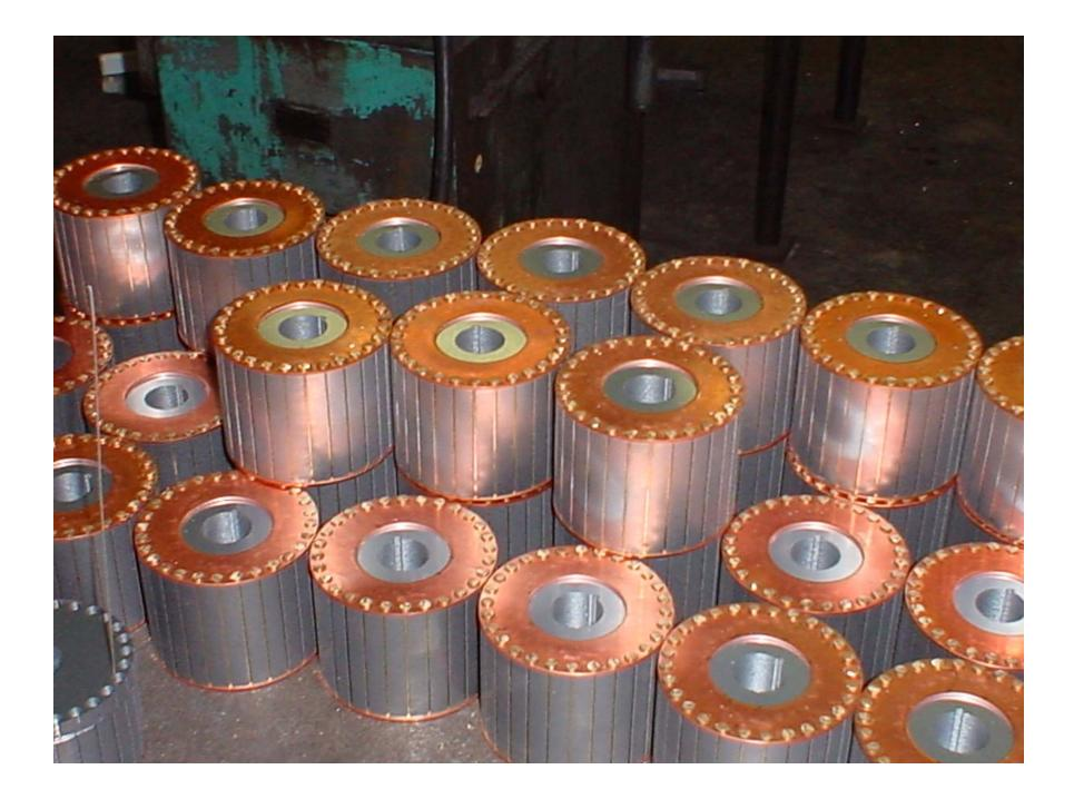
Speed and torque can be tailored to individual requirements by changing the conductivity of the rotor bars.
